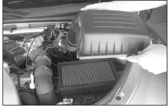
4. Unclip the upper air cleaner lid, then, remove the upper air cleaner assembly as shown.
